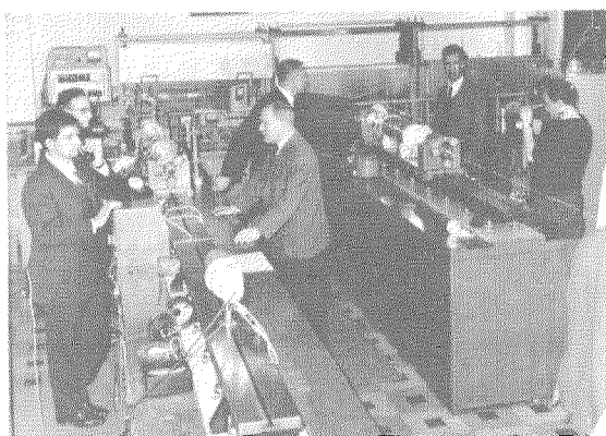
Figure 8—View of the Laser Research Laboratory of Laboratoire Central de Télécommunications just before the television presentation. The laser at the left was used for speech transmission while the more powerful unit to the right projected a laser beam on a wall outside the laboratories.
