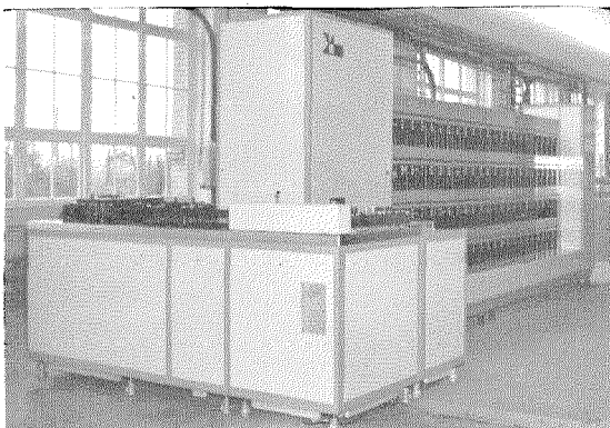
Figure 13—Automatic letter-sorting machine that reads 4-digit code numbers and sorts to 100 destinations.
