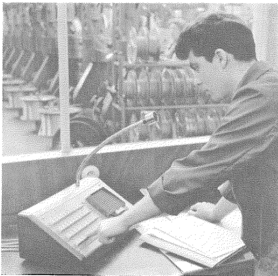
Figure 9—Master station of Dirigent 2/80 industrial intercommunication system.
