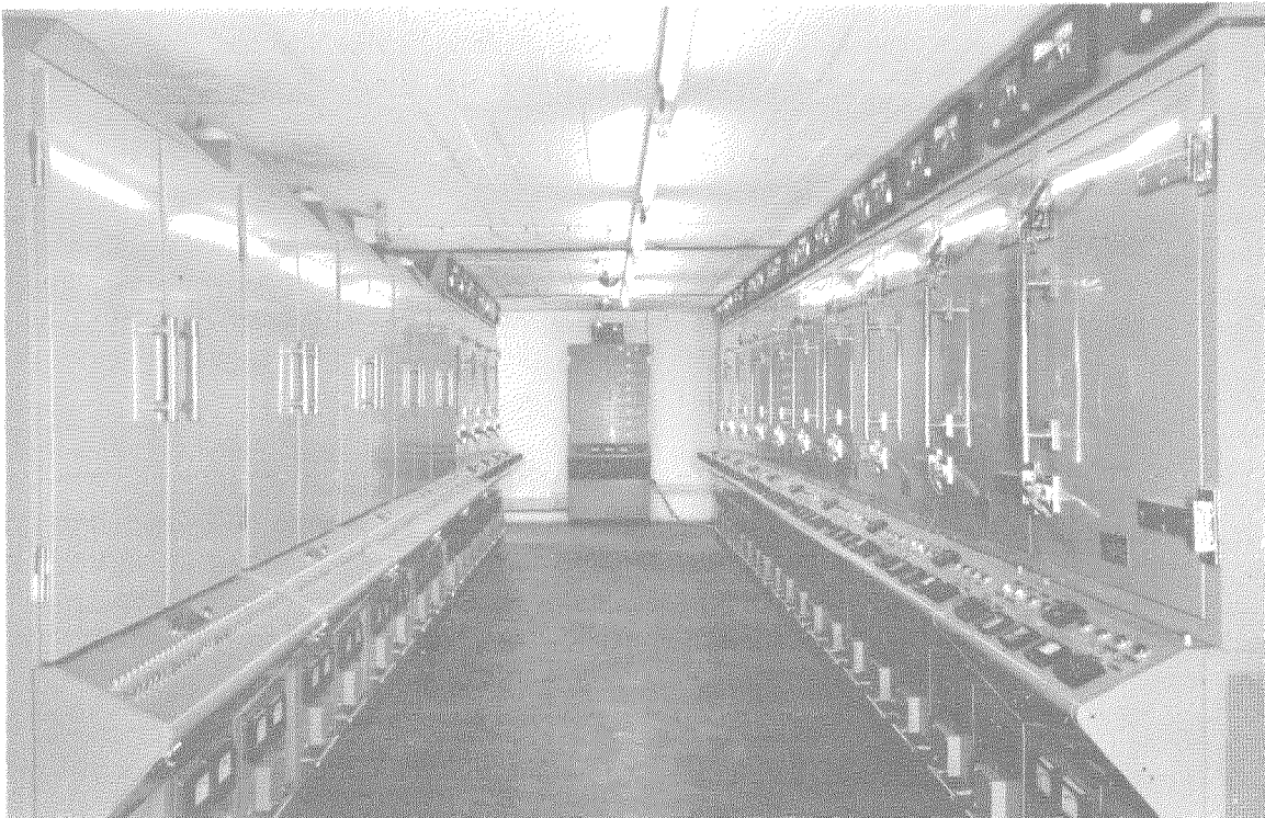
Figure 9—In this room 19 temperature-stabilized ovens are used to test components in extreme environmental conditions.
