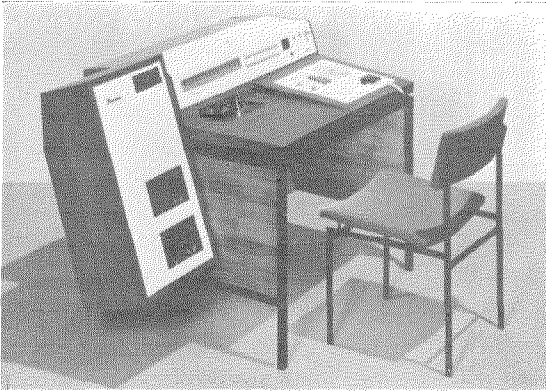
Figure 9—Standard Elektrik Lorenz document encoder.
