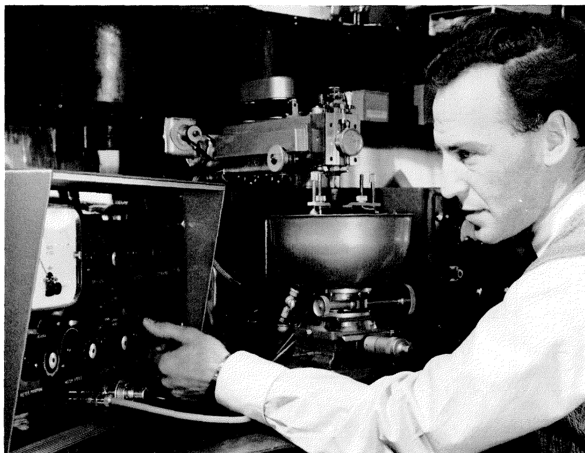
Figure 12—Equipment for machining to extremely close tolerances by spark erosion, built as a research tool to facilitate a study of the physics of erosion and to establish the ultimate limitations of the process. Individual spark discharges, occurring at high frequency, remove micron-size particles without physical contact between the electrode and workpiece contained in the bowl. The machine is being used in the construction of millimetre-wave tubes and components, thin-film evaporation masks for microcircuits, and the direct machining of semiconductor materials.
