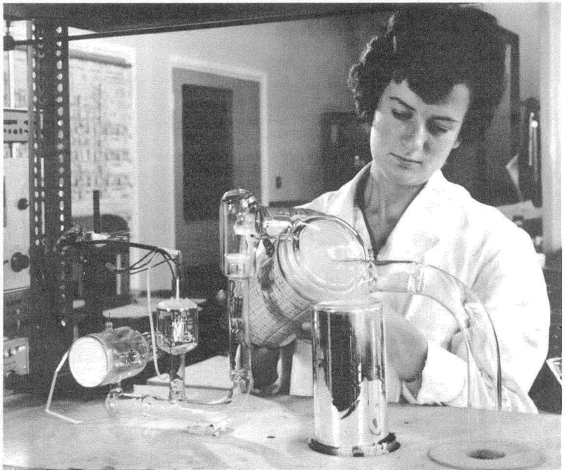
Figure 11—A field-emission microscope used in the study of semiconductor surfaces. This equipment enables an image of the surface of a fine point of the material under investigation, magnified some 100 000 times, to be observed on the fluorescent screen (seen on the extreme left). The liquid air being poured into the Dewar flask is to maintain an ultra-high vacuum ( 10^{-9} torr) within the system. The glass-work is of special construction required for ultra-high-vacuum studies.
