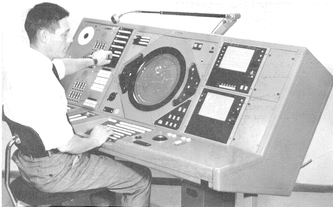
Figure 2—Control desk with indicator in place.
