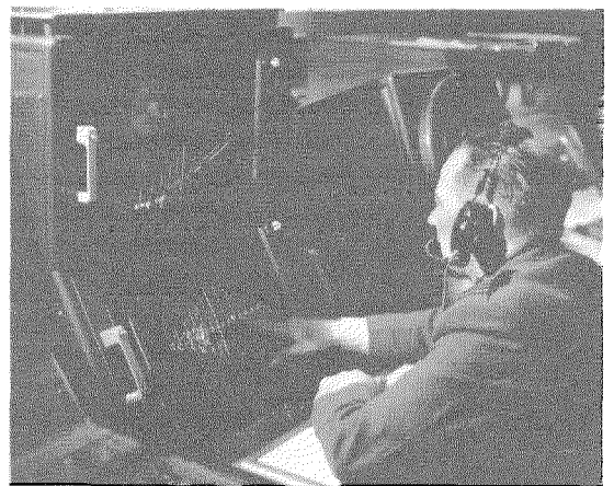
Figure 7—Display console of the SLA-3C precision approach radar.
