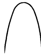
Figure 5—The sum of all 4 inputs, A + B + C + D , is used for the communication channel and also for tracking. When it is multiplied by the difference pattern of Figure 4 in a detector, a direct-current error voltage is produced.
