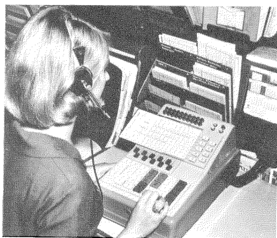
Figure 8—Push-button set in New York for making airline reservations in London via transatlantic telephone cable.
