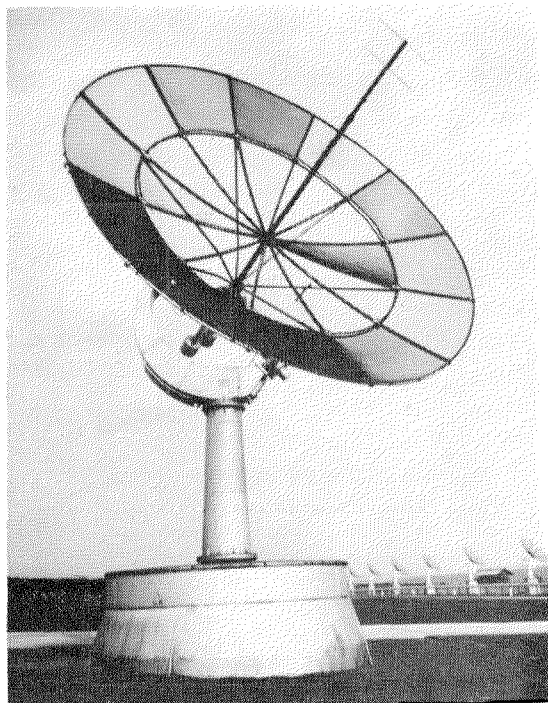
Figure 5—Paraboloidal antenna and in background part of 48-antenna array used for radio astronomy at the Humain field station of the Belgian Royal Observatory.
