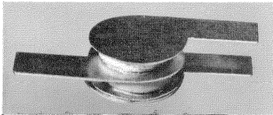
Figure 1—Matched pair of germanium tunnel diodes coded type JK60A.
