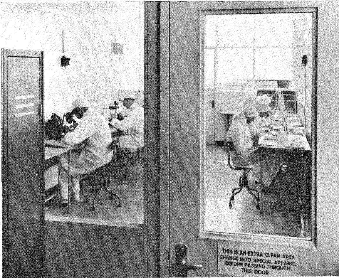
Figure 1—Typical extra-clean area for assembly of components.
