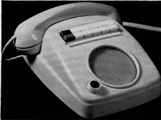
Figure 6—Dirigent master station for working with 10 substations in the star connection. The substations cannot communicate with each other.
