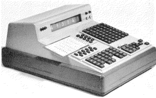
Figure 22—Load-control set used in the weight and balance system installed at Copenhagen-Kastrup airport for Scandinavian Airlines.
