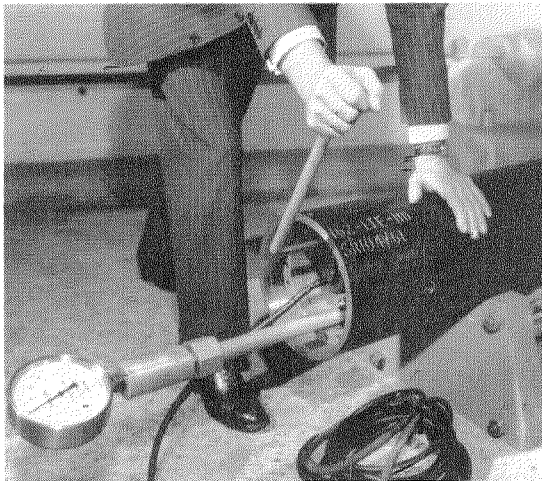
Figure 2—Measuring device showing pressure of petroleum-jelly seal. Neither pressure nor jelly is lost in connecting the device or in making a measurement so measurements may be repeated at any time without penalty.
