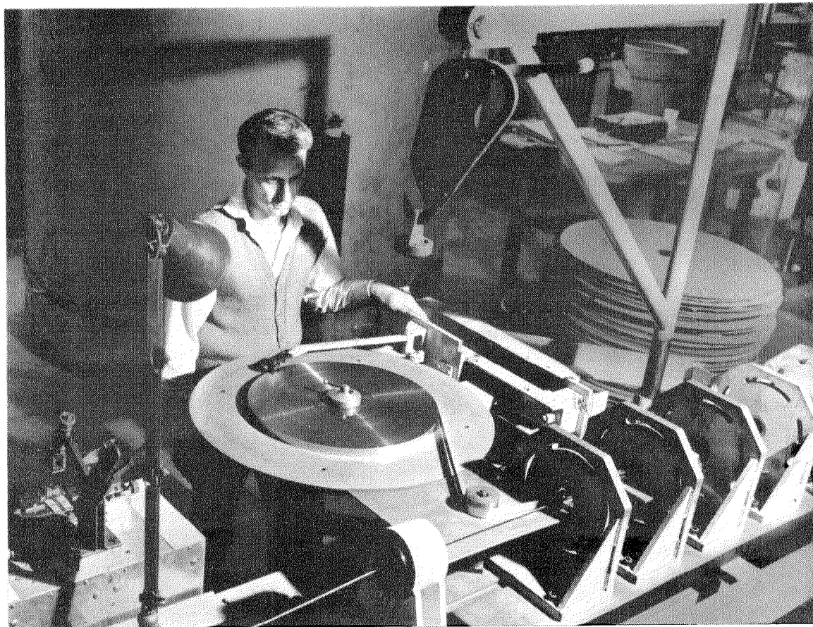
Figure 3—Box seaming machine. A 19-strand steel wire and a flat copper tape pass through 10 pairs of shaping rollers, some of which are visible at the lower right, to shape the tape round the wire and form a box seam to secure it.
