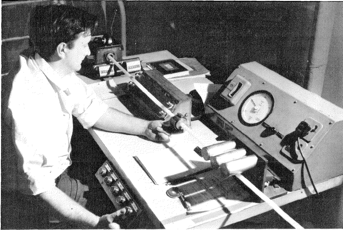
Figure 7—The completed core is examined at this inspection bench, where it can be stopped at will to check for faults indicated on the charts from the extruder measurements. A light box is used to inspect for inclusions or impurities in the polythene.
