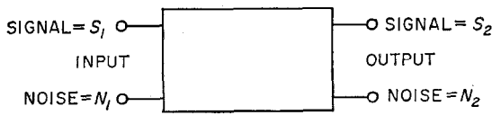
Figure 12—General two-terminal pair network.
