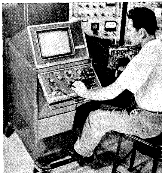
Figure 10—Precision oscilloscope using 14-inch (36-centimeter) cathode-ray tube.
