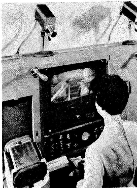
Figure 2—Tellers position for the autobanker. Closed-circuit television, an intercommunication sound system, and a pneumatic-tube to transport papers and money eliminate the effects of distance and permit transaction from a remote drive-in window of all banking services that are normally handled by a teller in the bank.
