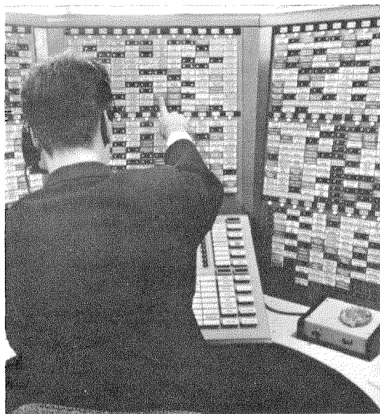
Figure 2—Part of the Doris consol for the Direct Order Recording and Invoicing System utilizing pre-recorded data and punched tape for the full processing of orders.
