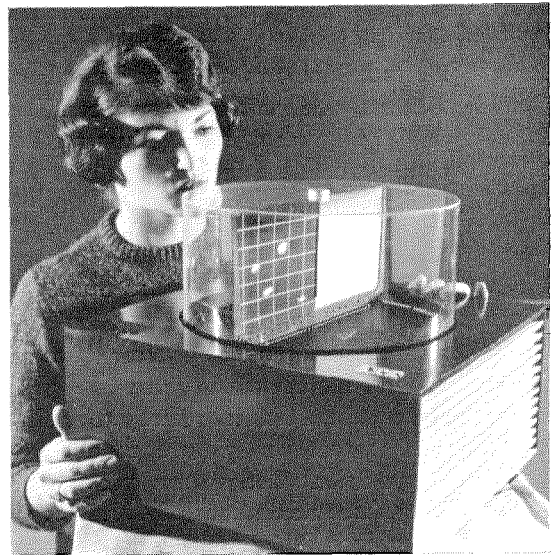
Figure 7—As the screen rotates rapidly about its vertical axis, a short-duration pulse of light from a cathode-ray tube illuminates a spot on it which, through synchronous operation, appears to stand still in three-dimensional space.
