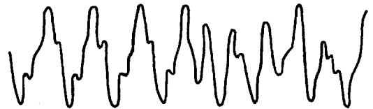
Figure 20—Oscillogram of response to code group 0000000011010100 transmitted at 2000 bauds.
