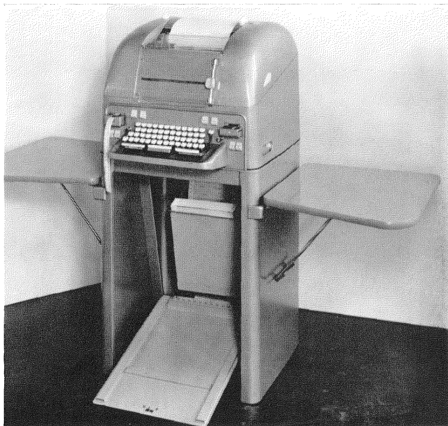
Figure 2—Page printer mounted on a pedestal showing magazine for handling message blanks in folded strip form mounted within the pedestal.
