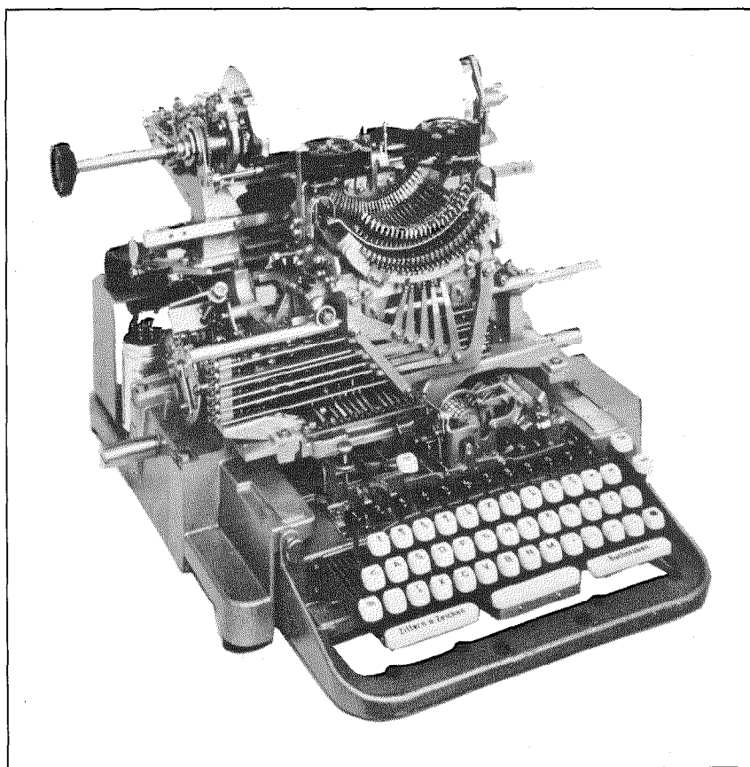
Figure 1—Teleprinter for reliable transmission of numbers. The set of black keys used in the third-shift position is visible above the conventional keyboard.
