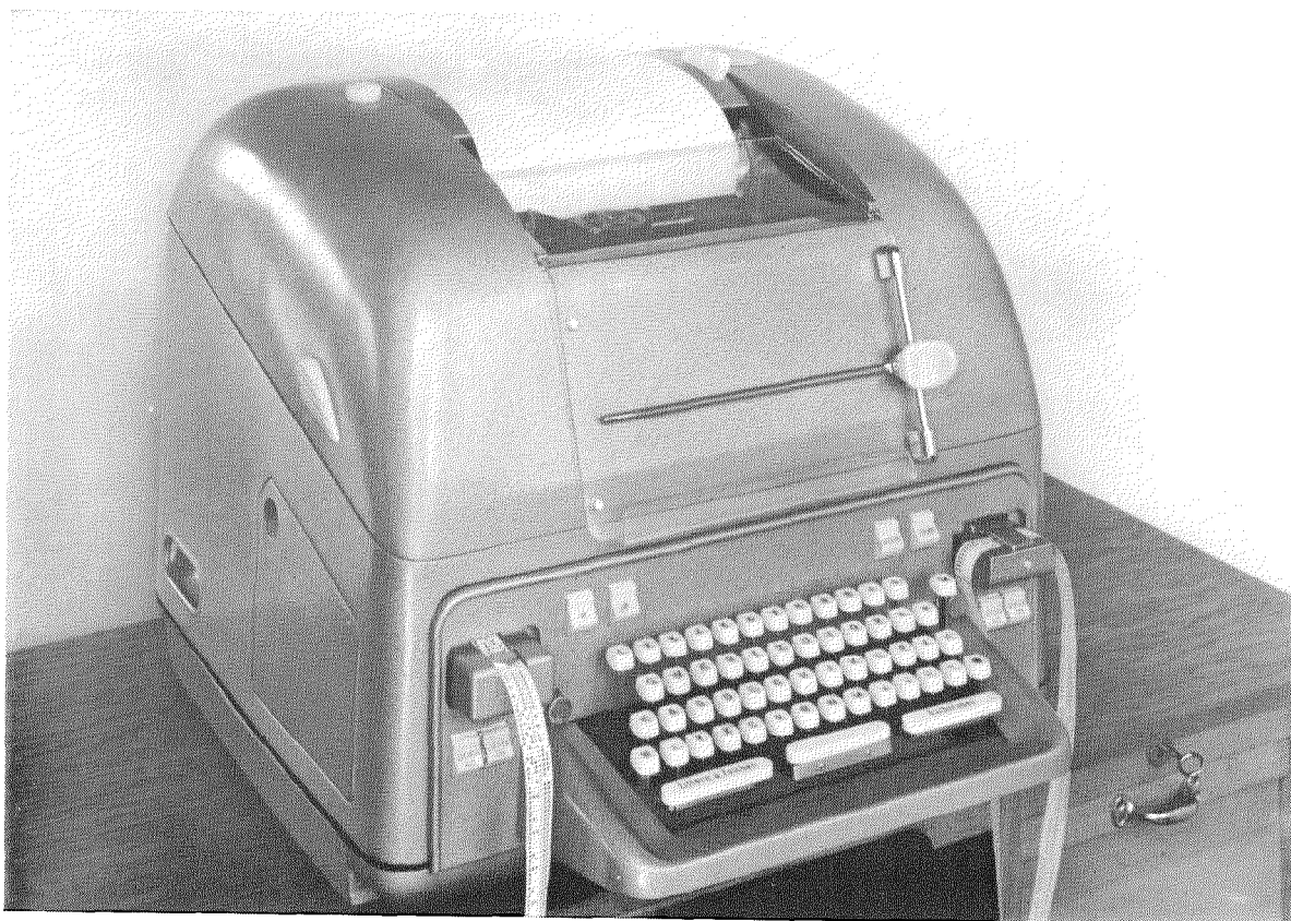
Figure 1— LO-15-B page printer with built-in reperforator and tape transmitter mounted on a desk.
