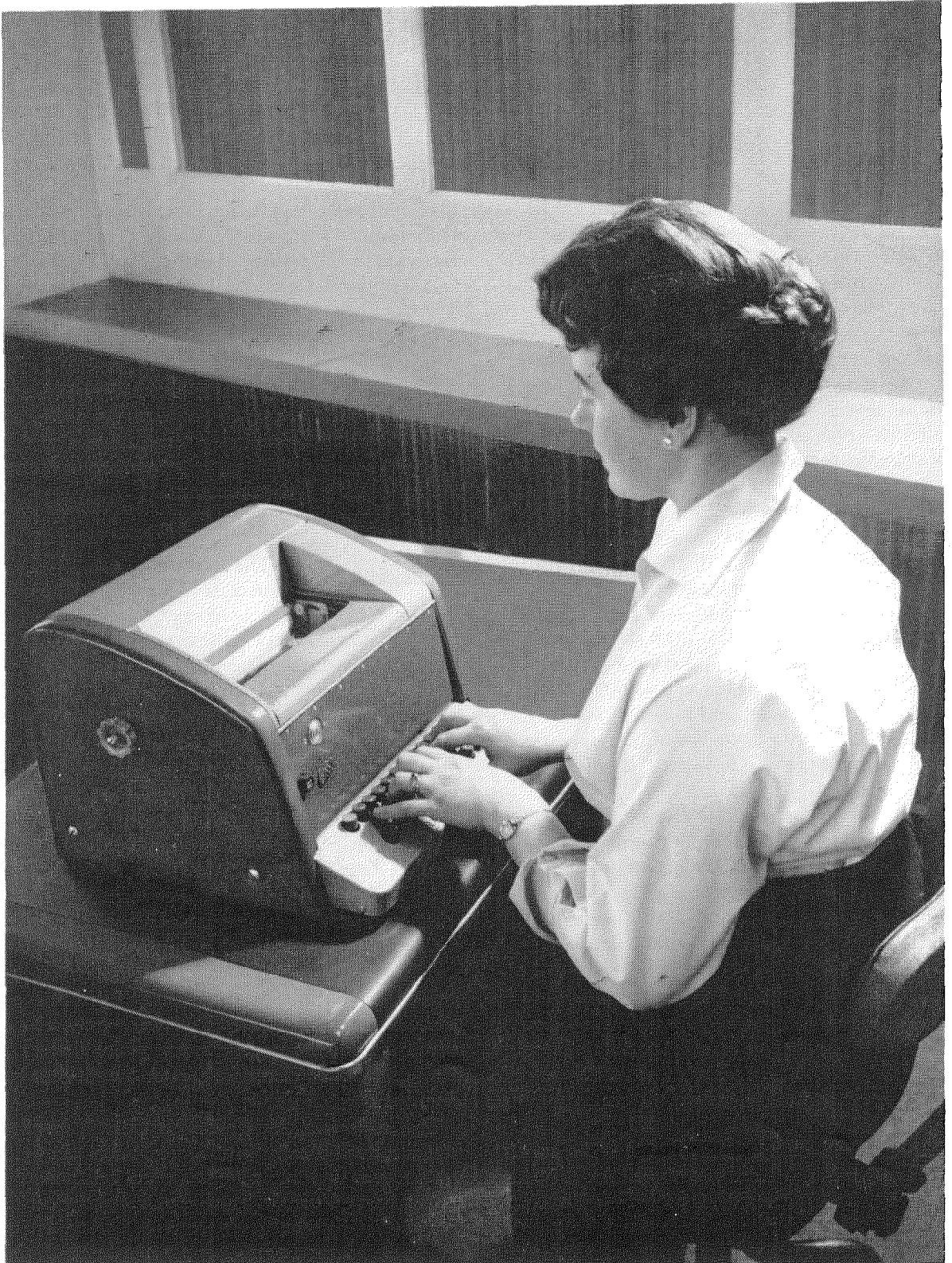
Figure 1—Smaller, lighter, and simpler than any other teleprinter in production in the world, the model Seventy-five is capable of sustained operation at 100 words per minute with high standards of attention-free performance.
