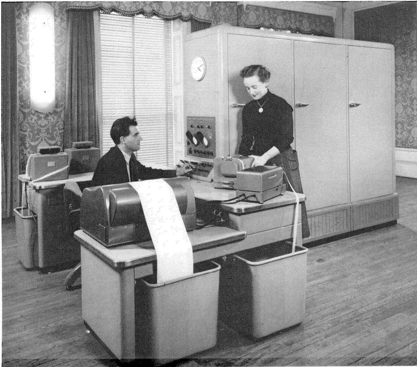
Figure 3—Application of teleprinter equipment to record output data from an electronic digital computer in punched-tape and printed-page form.
