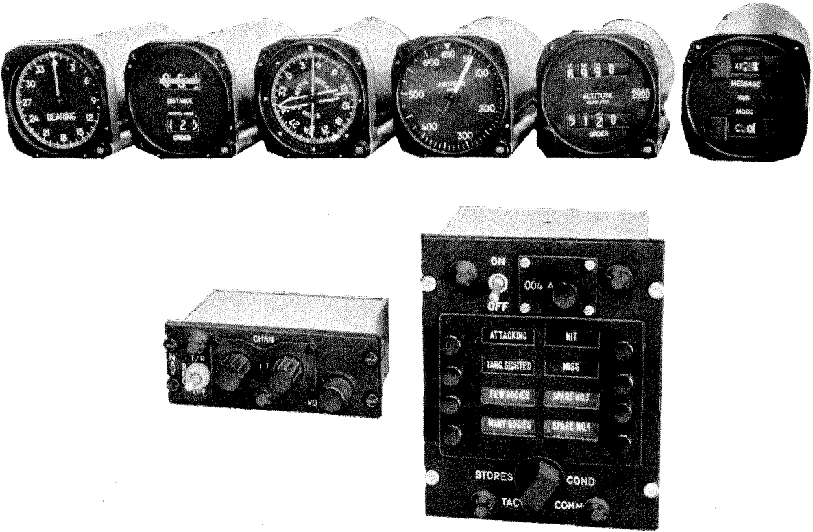
Figure 4—Controls panels for AN/ARN-26 and AN/ARN-21 and instrument group for the AN/ARN-26.
