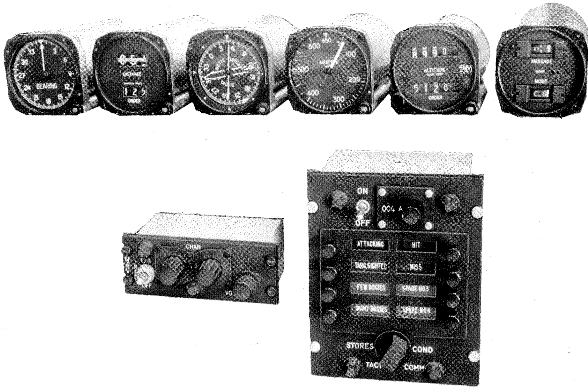
Figure 3—Top row shows bearing, distance, radio-magnetic-compass, air-speed, altitude, and ready-made-message indicators. Below is the control box and the panel for sending ready-made messages.
