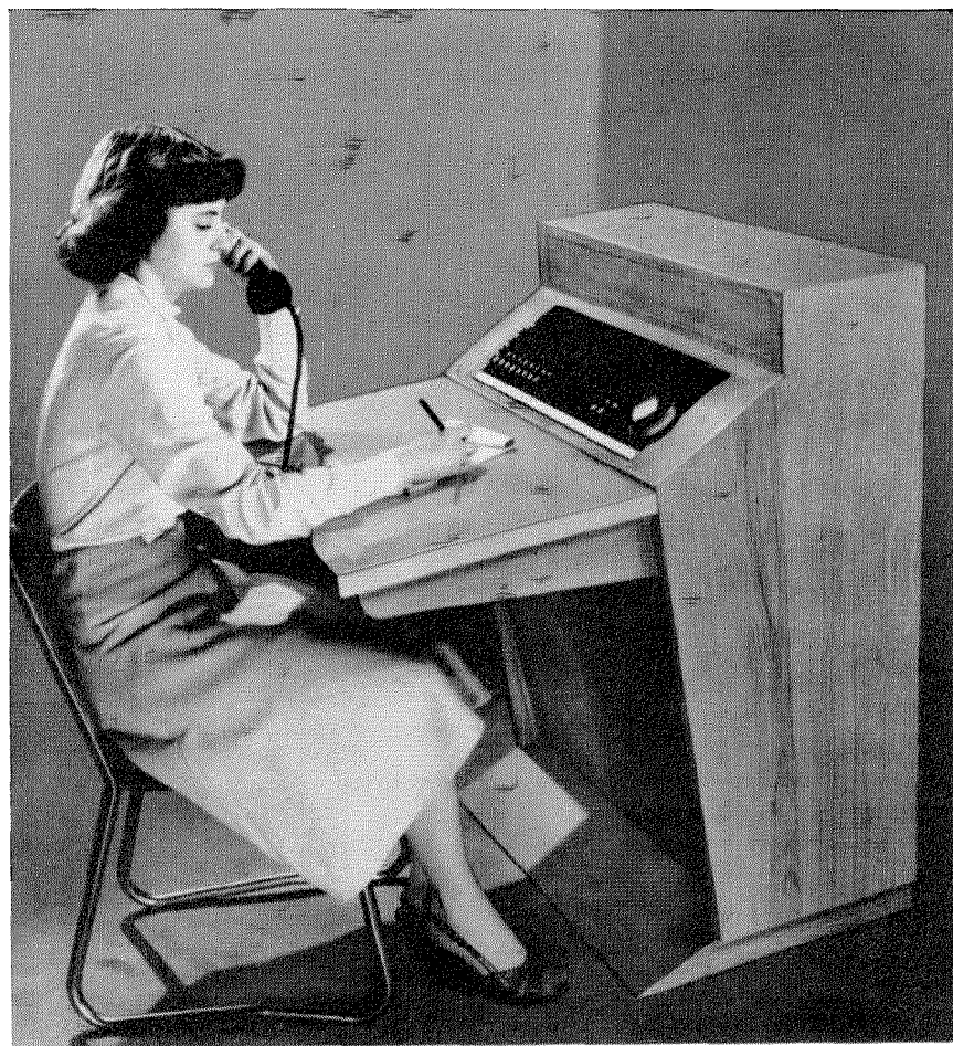
Figure 11—Operator's position handling up to 16 trunks and 2 operator's lines.
