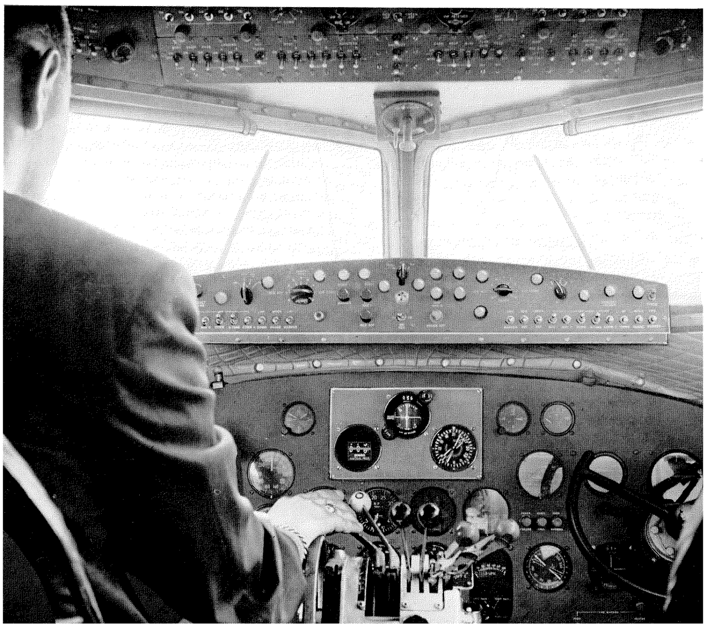
Figure 3—In the pilot's compartment, the left meter gives distance and the center and right meters give bearing.
