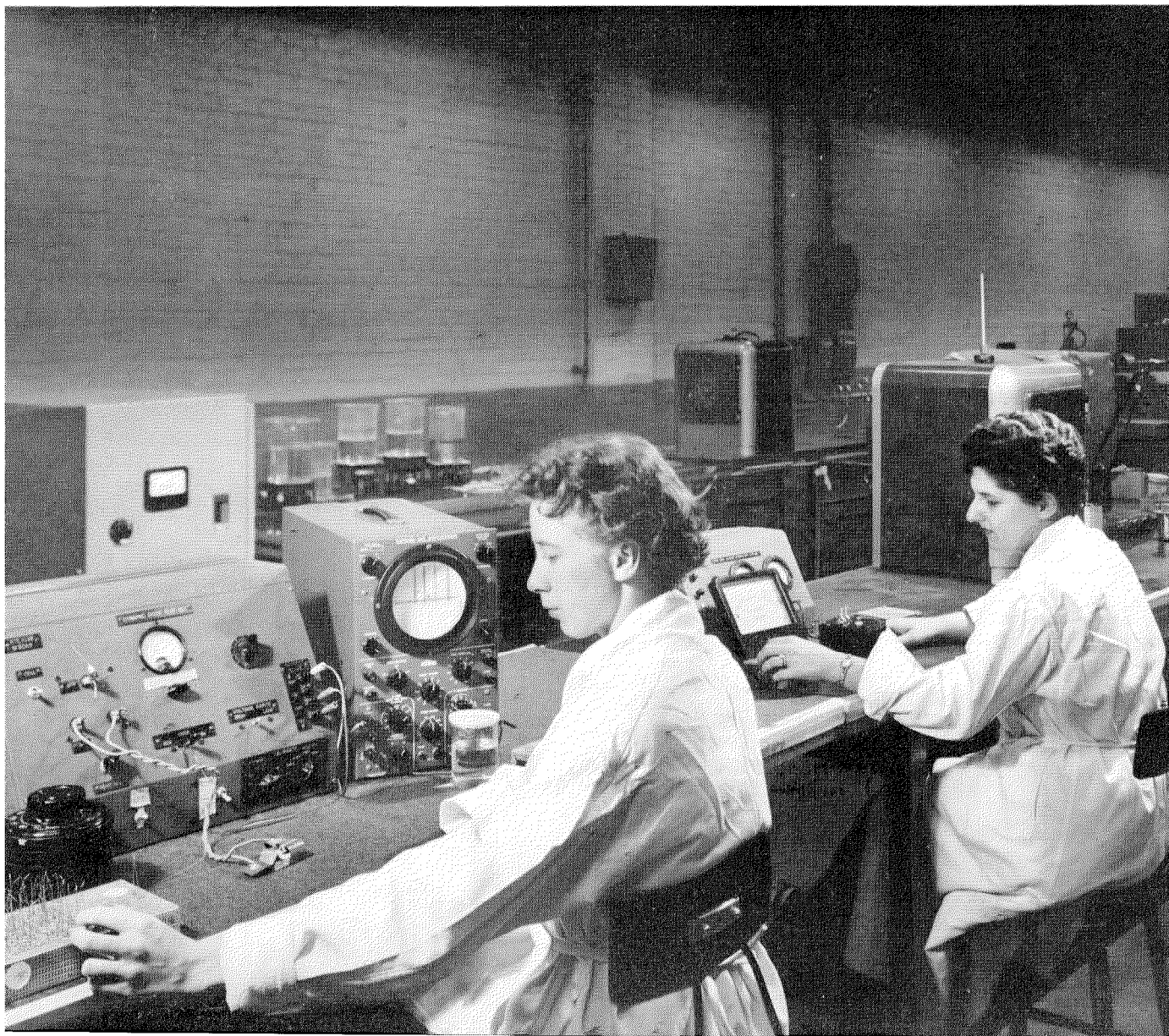
15. Characteristics of the diodes in the forward- and reverse-current directions are made at the two positions shown here.
