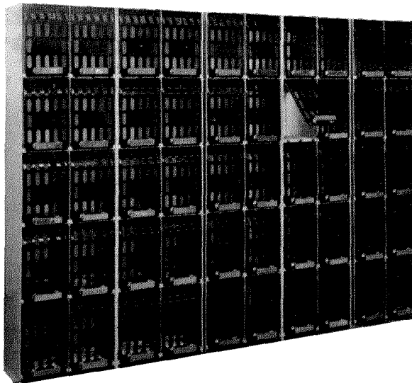
Figure 8—Destination cases to which the mail is distributed. They may be unloaded while sorting is in progress.
