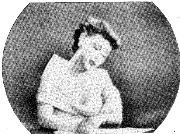
This mild form of interference may be caused by radiation from an inadequately shielded oscillator in a nearby television receiver. Interference from a radiotelegraph transmitter, while similar, will be influenced by keying, whereas that from another receiver changes only slowly.
