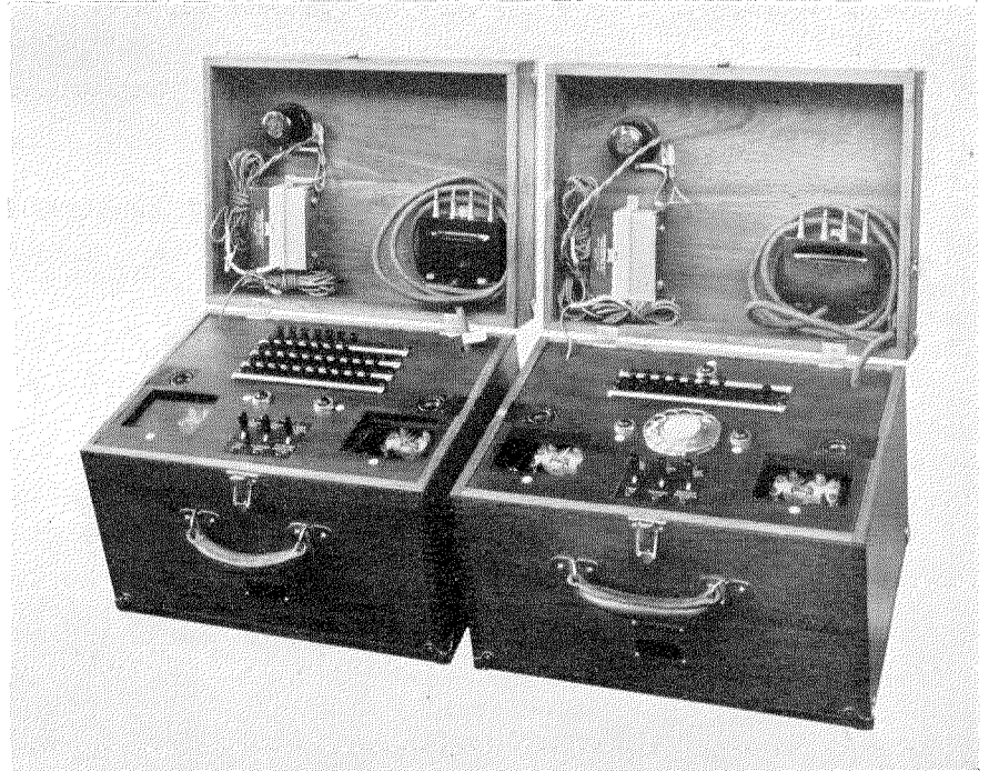
Fig. 13—Portable sets for routine tests are usually supplied in pairs, one for use at the central control point; other is for use at substation.
