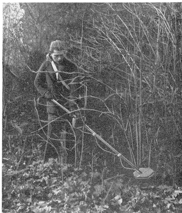
Mine detector DM-3 in operation over difficult terrain.
