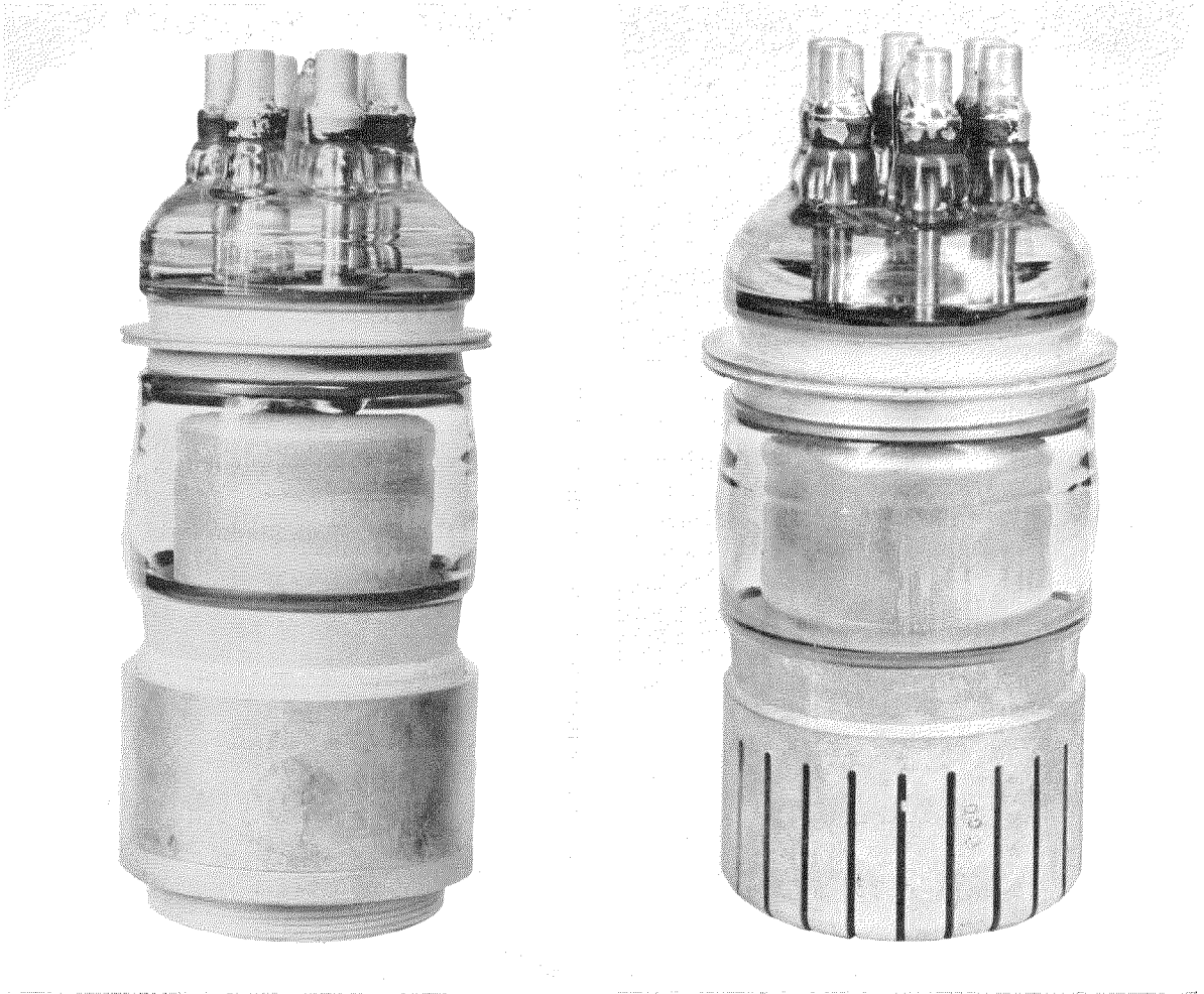
Fig. 32—8C23 with (left) and without (right) water jacket.
