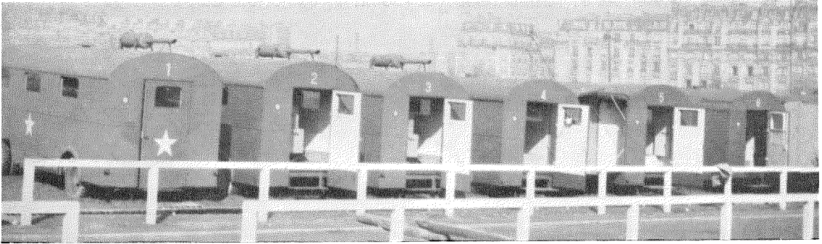
Fig. 6—Six of the 17 trailers in which “Sig Circus,” the 60-kilowatt mobile radio station, is housed may be seen above. Facilities are included for 200 000 words daily of radiotelegraph traffic, complete broadcast transmission including a studio and control booth, as well as facsimile transmission and reception, and wire, film, and disk recording.
