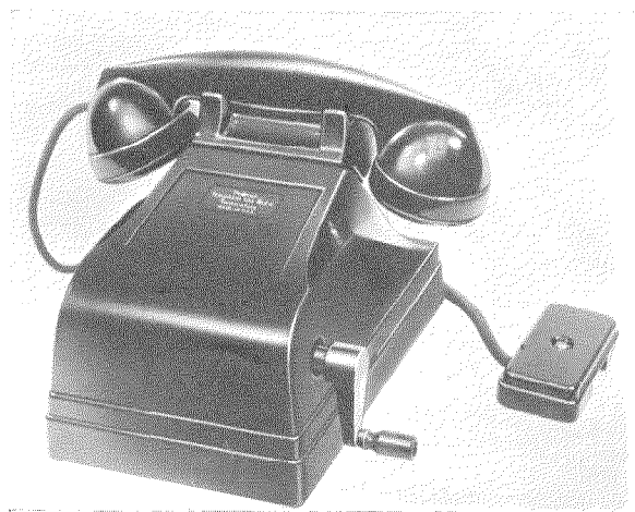
Fig. 14—Convertible magneto telephone. The cradle may be reversed to convert it to a wall-type instrument.
