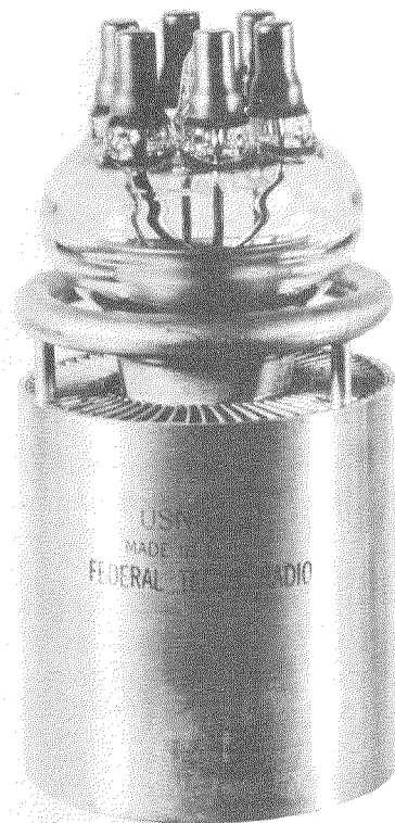
Fig. 32—7C23 forced-air-cooled triode used in radar service.
