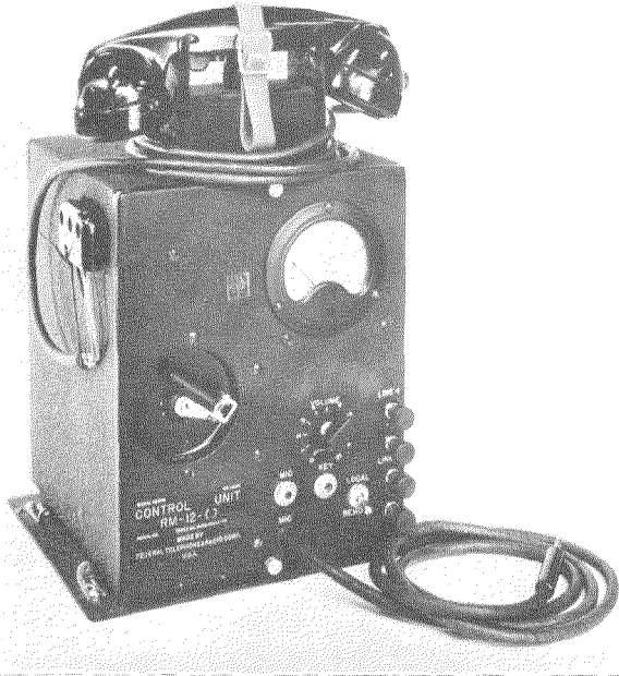
Fig. 16—Equipment used at a radio transmitter to be controlled from a remote position. This apparatus operates with that shown in Fig. 17.
