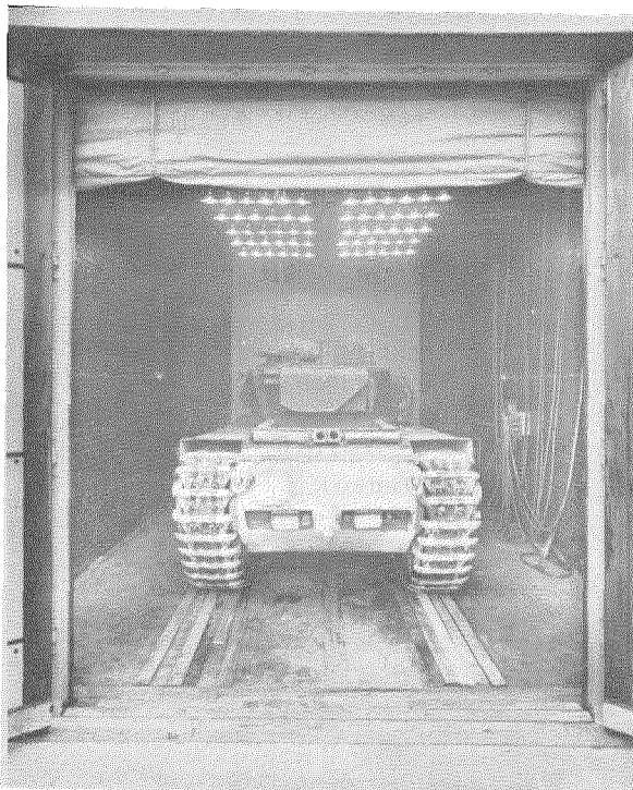
British Army tank in one of the S.T.C. tropical test chambers. In one month, the equivalent of two years service under extreme conditions of heat and humidity such as are encountered in tropical climates may be simulated.
