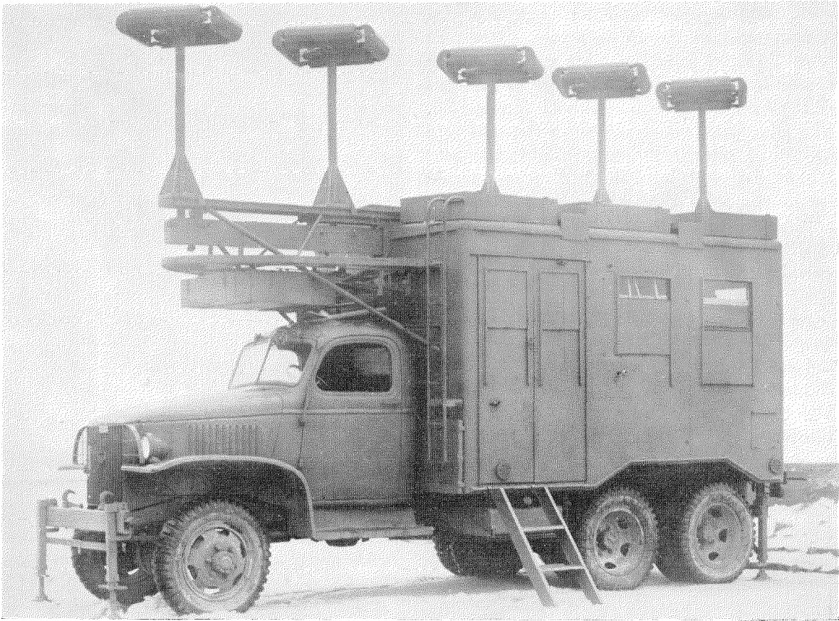
Army-type mobile localizer, SCS-51, manufactured by Federal Telephone and Radio Corporation. The antenna array consists of three main radiating loops and an auxiliary pair to increase the course sharpness.
