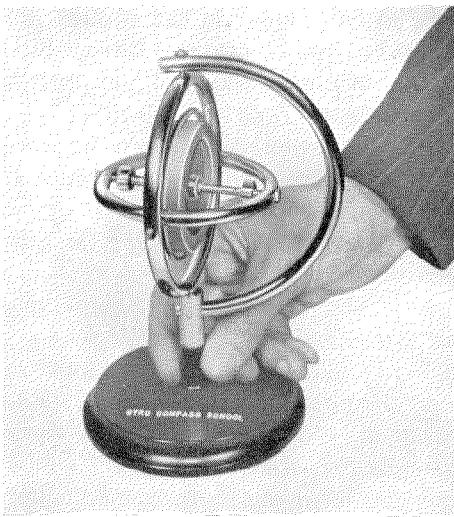
Fig. 6—When spinning, the gyro exhibits "gyroscopic inertia."
