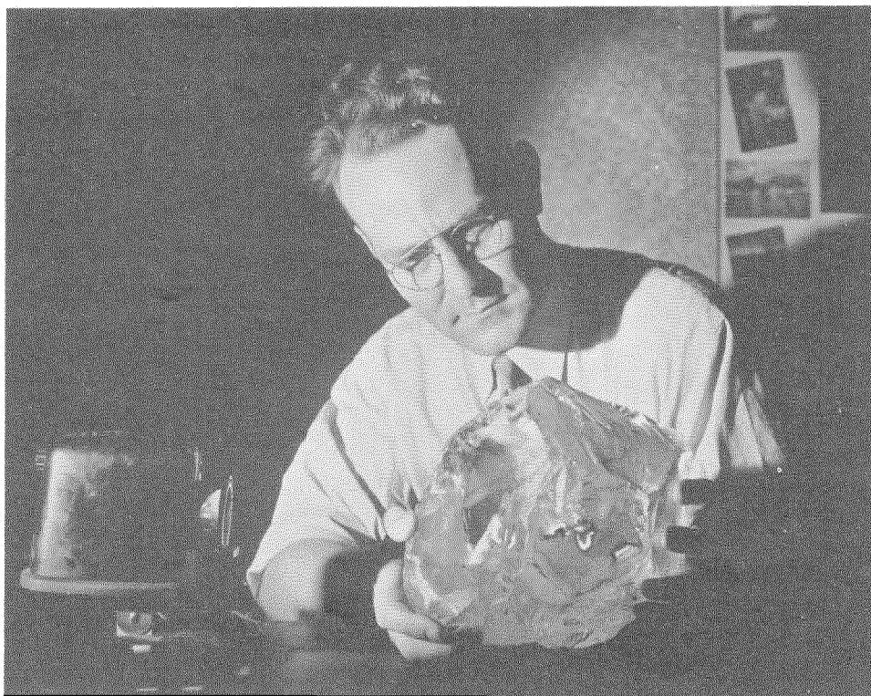
Fig. 7—Examining a Large Piece of Raw Quartz for Flaws Prior to Processing it at the Federal Telephone and Radio Corporation Crystal Laboratories in Newark, New Jersey.
