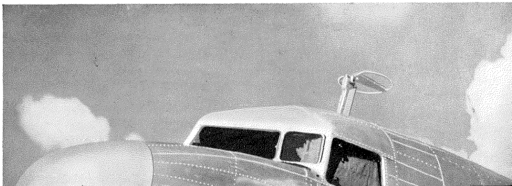
Fig. 10—U.H.F. loop antenna of Type II installed on a transport 'plane.
