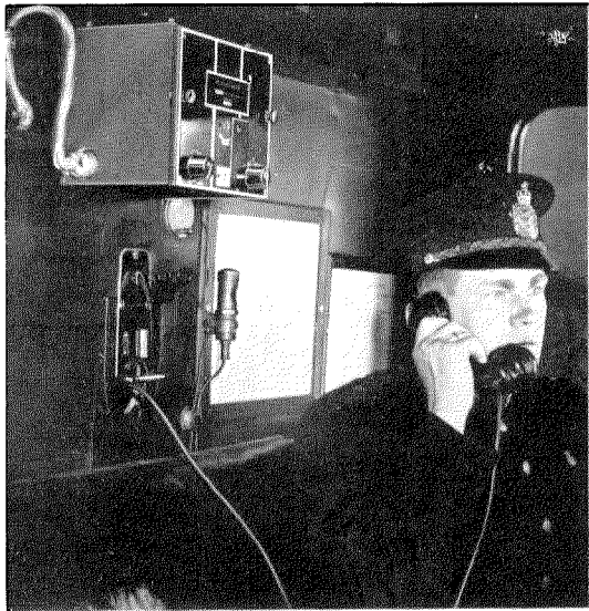
Fig. 5.B.—Receiver and Control Unit in Transport Car.
