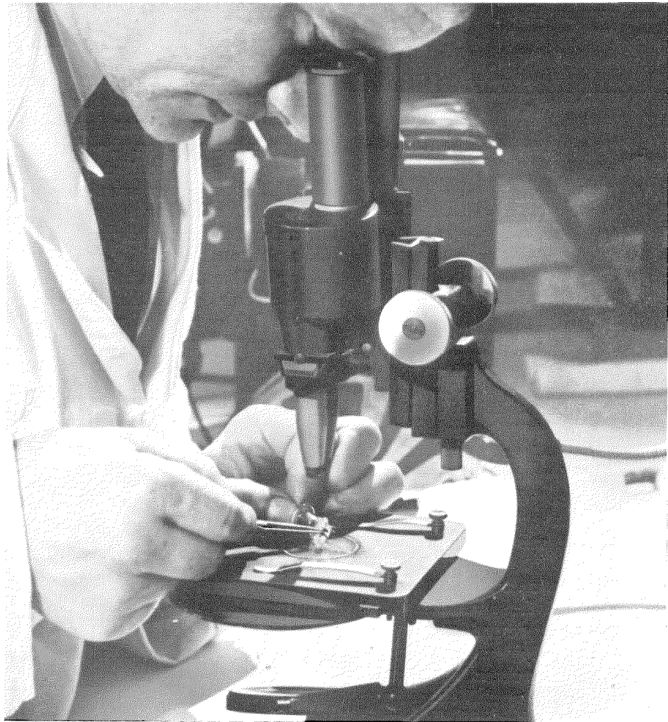
Assembling a centimetre-wave tube having an anode with a radius of eight-thousandths of an inch. Because of its small size, this type of tube is assembled under a binocular magnifier. (Les Laboratoires, L.M.T., Paris.)
