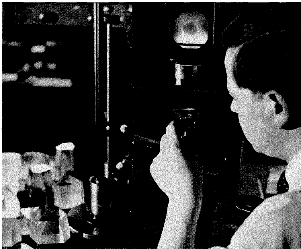
Illustrating method of controlling the perpendicularity of a quartz crystal by means of polarised light, resulting in the formation of "airy" spirals—Les Laboratoires, Le Matériel Téléphonique, Paris.
