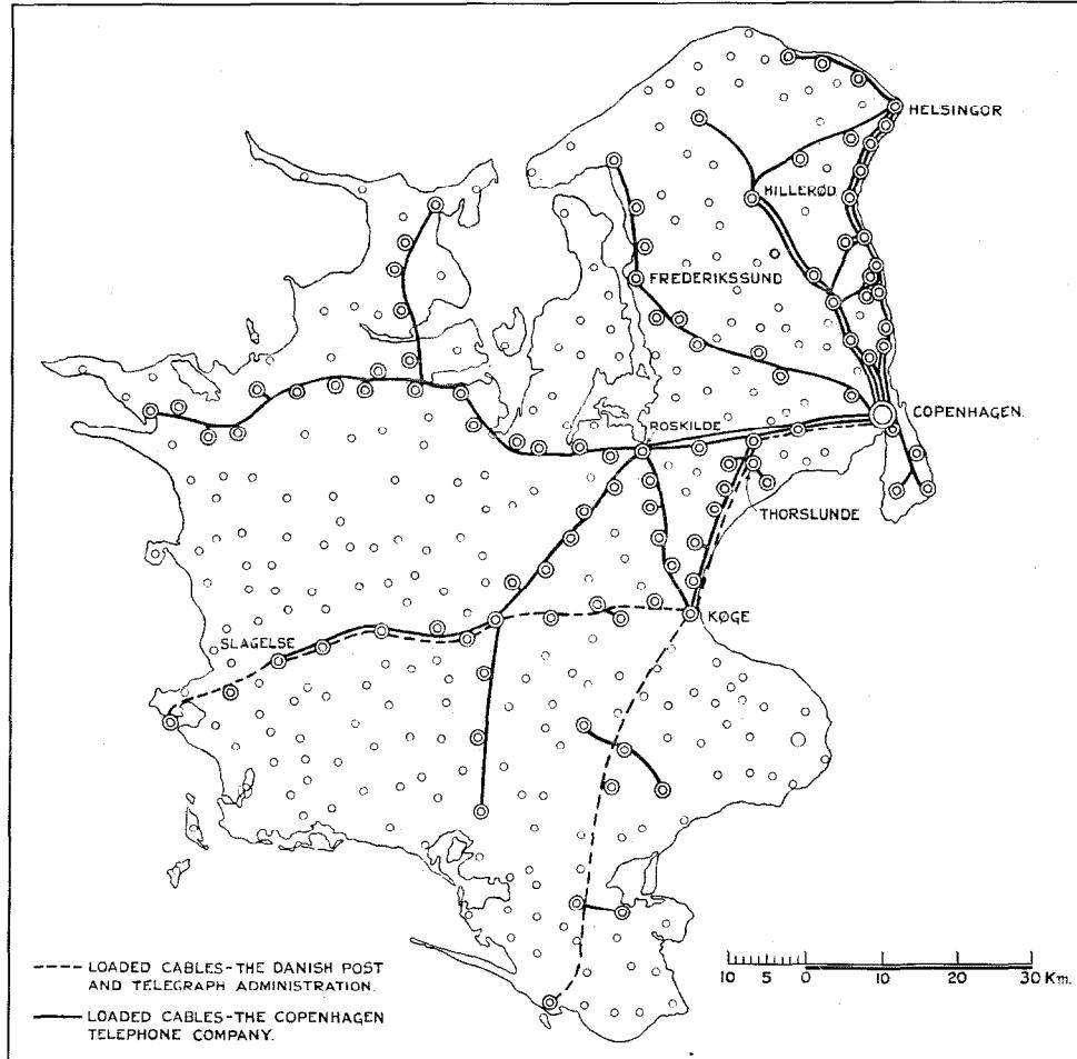
*Figure 1—Loaded Cables of The Danish Post and Telegraph Administration and The Copenhagen Telephone Company.*
