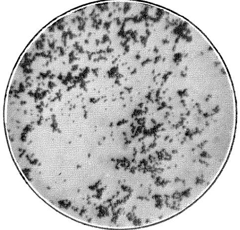
Figure 13—Iron Powder (Deposited from Iron Carbonyl)  $\times 75$ .
