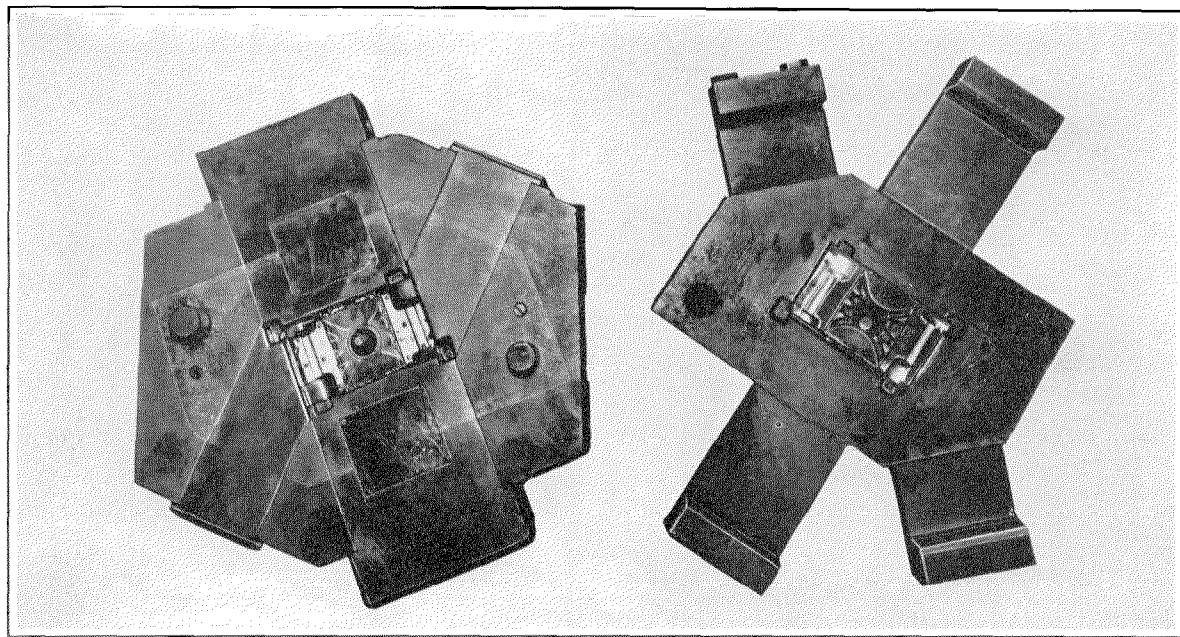
*Figure 6—Mould for Brush Carriage shown in Fig. 5.*
