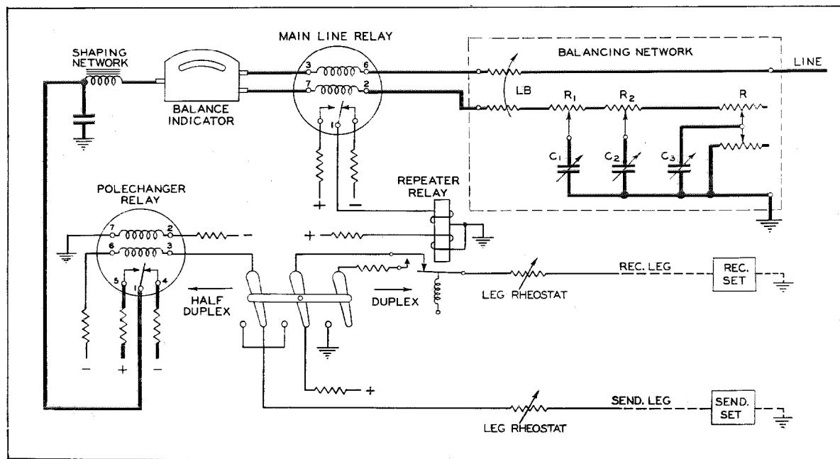
Figure 4—Differential Duplex Terminal Set Schematic.
