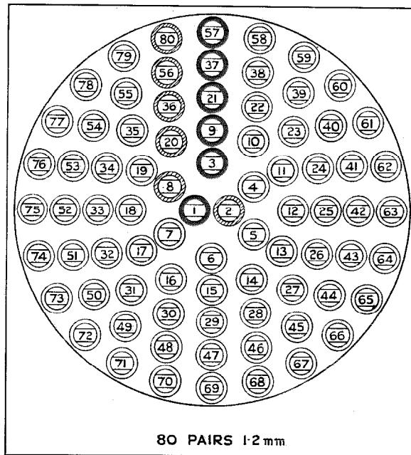
Figure 3—Cable Profile—Coil Loaded Thorslunde-Køge Cable.
