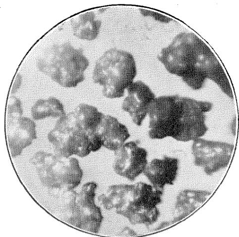
Figure 11—Aluminium Powder (By Stirring Molten Metal)  $\times 50$ .
