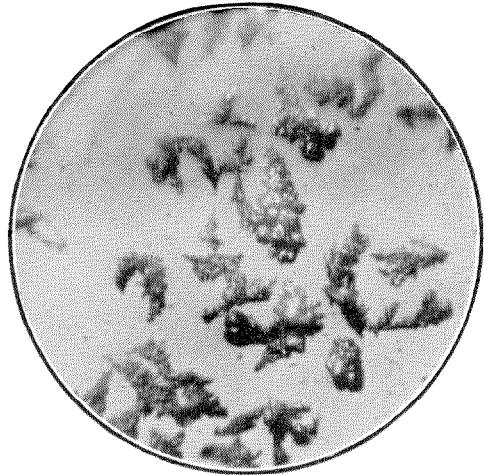
Figure 12—Copper Powder (Electrolytically Produced)  $\times 40$ .
