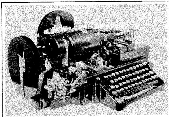
The attachment may be switched in and out of use by the operation of a lever, and if no local record is required when perforating tape, the keyboard transmitter can be cut out. In the latter case the perforator cam is released from the code shaft of the transfer unit instead of from the transmitter shaft, and the maximum average speed at which the keyboard can be operated is thereby increased from the normal speed of 420 characters to 840 characters per minute.
