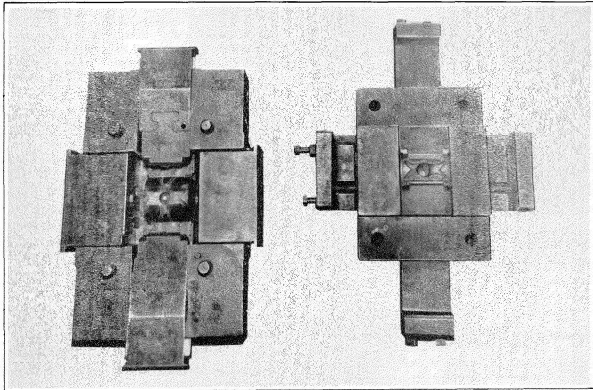
Figure 4—Mould for Selector Frame shown in Fig. 3.
