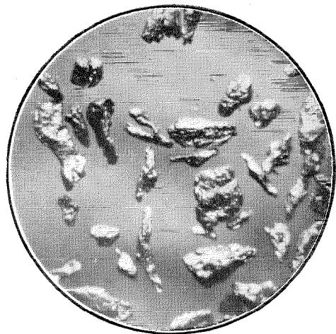
Figure 7—Iron Powder (Ground from Electrolytic Iron)  $\times 40$ .
