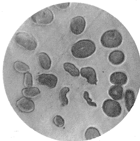
Figure 15—Cross-Section of Acetylated Mercerised Cotton Dyed with a Disperse Colour. Even Dyeing Indicates Even Acetylation. (Magnification of this figure approximately of the order of 600).
