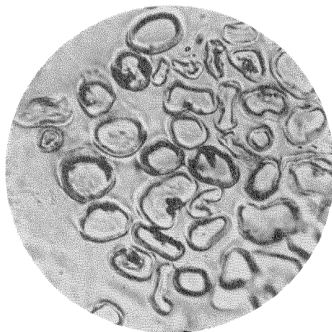
Figure 16—Cross-Section of an "Immunised" Cotton (Cellulose Benzoate) Dyed with a Disperse Colour. Only the Outer Ring is Coloured. (Magnification of this figure approximately of the order of 600).
