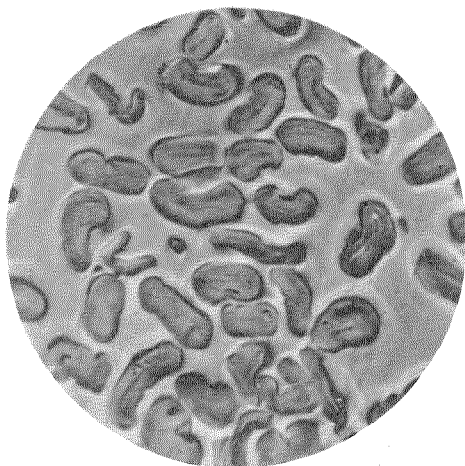
Figure 14—Cross-Section of Cotopa Fibres Dyed with a Disperse Colour. Even Dyeing Indicates Even Acetylation. (Magnification of this figure approximately of the order of 600).
