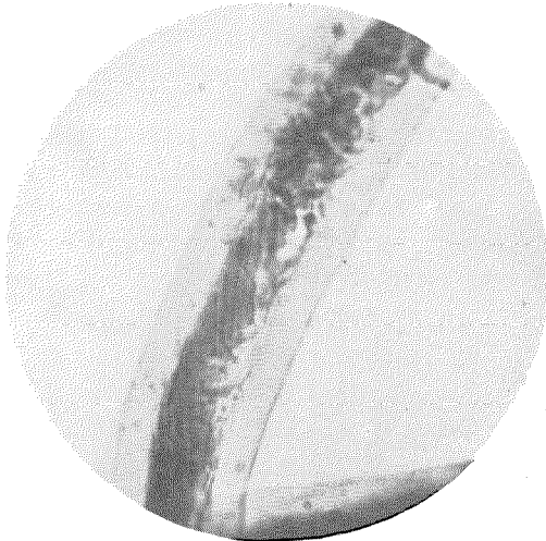
Figure 6—Part of a Cotton Fibre Showing Spiral Markings (Magnification 1000 X).
