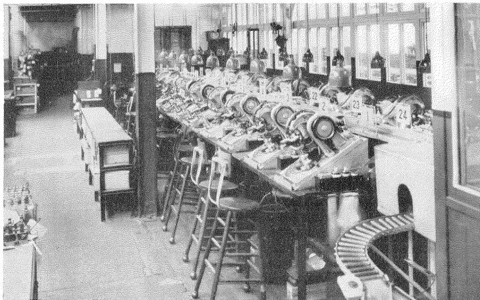
Figure 12—Coil Winding Room.
