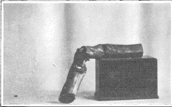
Figure 7—The Cable Crushed by Land Slips.
