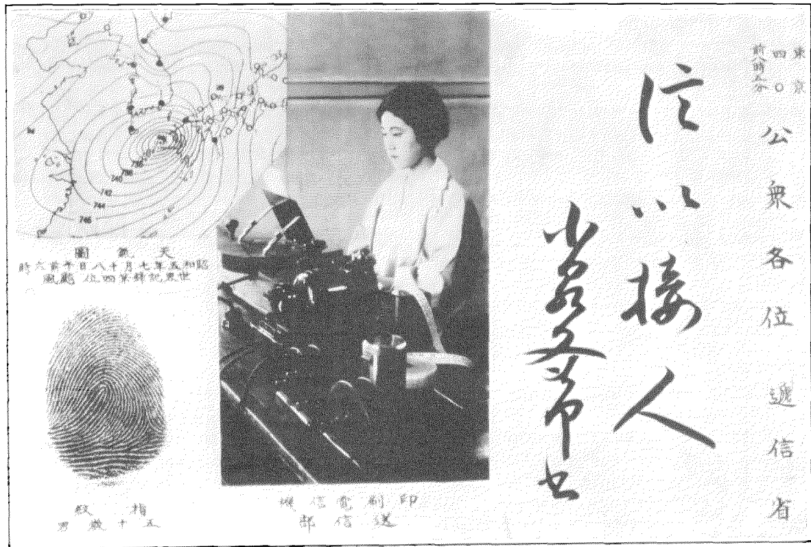
Specimen of Picture Transmitted Over Nippon Electric Phototelegraph System Between Tokyo and Osaka
