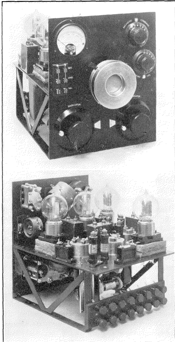
Figure 6—Condenser Transmitter Recently Developed by the International Standard Electric Corporation.
