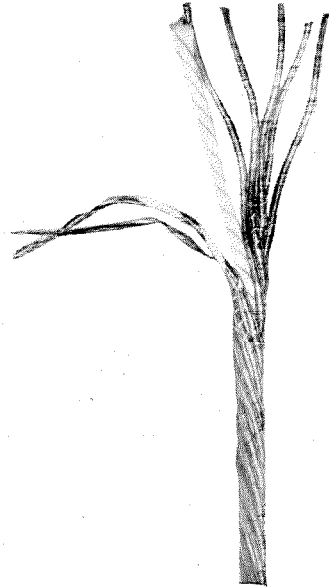
Figure 9—Enlarged View of Conductor S 3A Switchboard Cord
