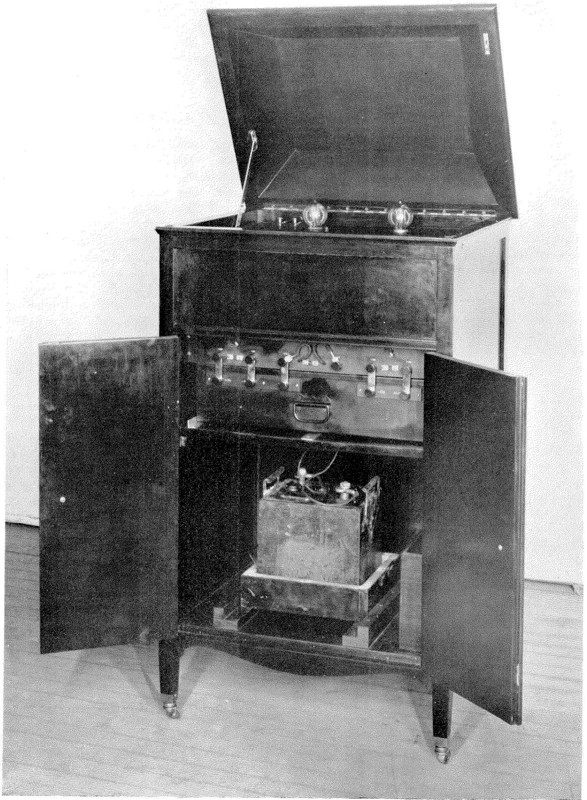
Figure 4—Amplifier for Condenser Transmitter-Cabinet
